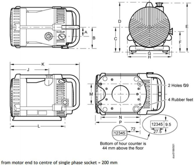
from motor end to centre of single phase socket = 2 from motor end to centre on/off = 124 mm Refer to Table 3 for dimensions
